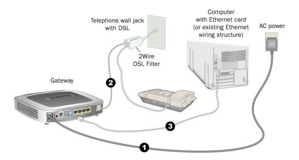
Figure 1. Gateway Connected Via Ethernet
